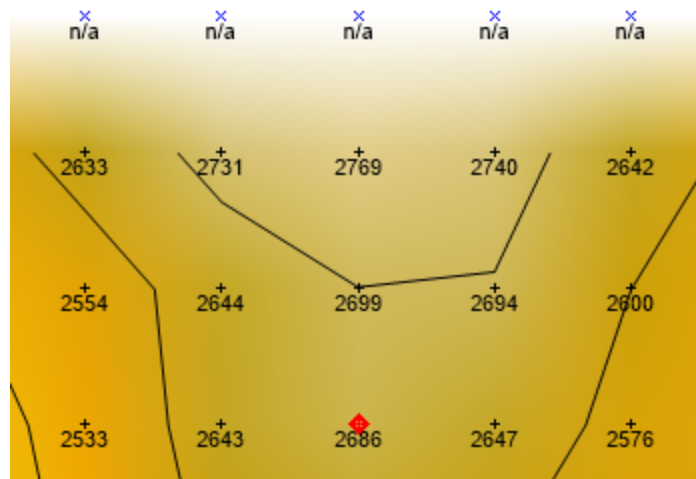
This image displays grid node symbols, labels, contour lines, and a color fill for a grid file.
