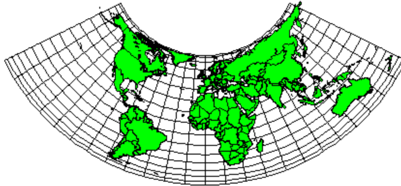
World Map Albers Equal Area Conic Projection Central Longitude: 0 Central Latitude: 0 Standard Parallel: 45 2nd Standard Parallel: 0
