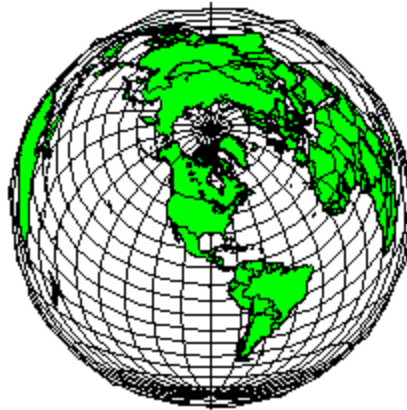
World Map Lambert Azimuthal Equal Area Pro- jection Central Longitude: -90 Standard Parallel: 45
