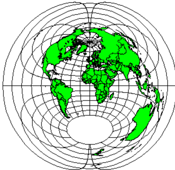
World Map Azimuthal Equidistant Projection Standard Parallel: 0 Central Longitude: 0
