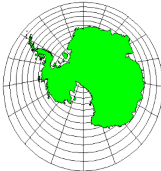
Antarctica Gnomonic Projection False Easting: 0 False Northing: 0 Central Longitude: 19.0 Standard Parallel: 2.4
