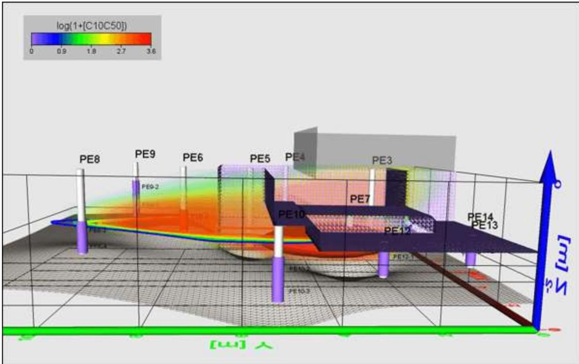
A grid file was generated in Surfer and imported into Voxler to represent the bedrock top detected at each boring location.
