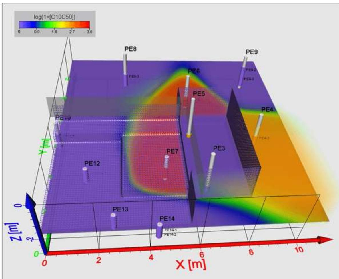
This Ortholmage module displays a 2D planar profile of contamination at a depth between PE6-3 and PE7-2.
