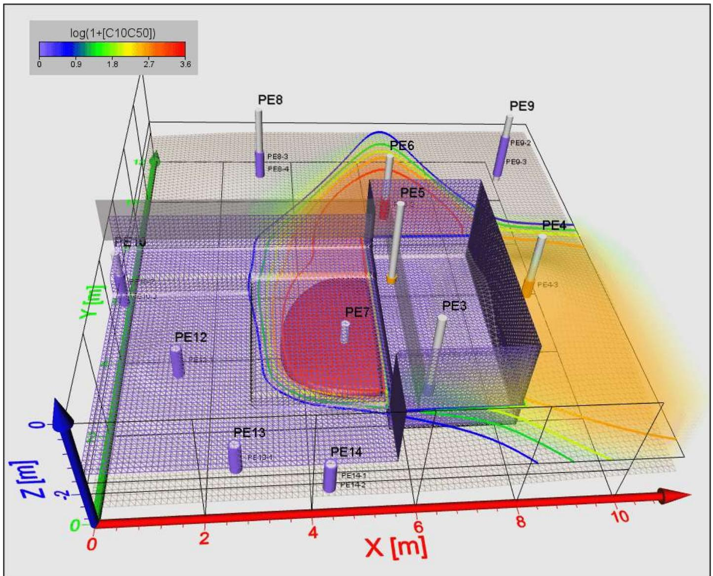
An orthographic view of the project. The leaking underground storage tank was removed from the PE3 and PE5 section and the contaminated bedrock was excavated. Thereafter, boring samples were taken from the surrounding area to determine the contamination plume. PE3 and PE5 were extracted from new soil which replaced the underground storage tank.
